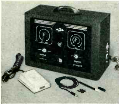
Electronic hair-removing setup consists of equipment shown. The foot-switch initiates automatically-timed pulses and controls length of manually-timed pulses
