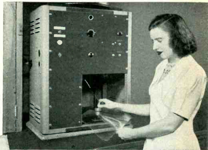
Inserting a sample preparatory to a voltage breakdown test. Kodapak Laboratory, Rochester, N. Y.
