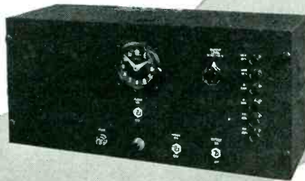
TYPE 2121A. LAB. STANDARD Outputs, 60 cycle, 0-110 Volts. 120-240 cycle impulses. Input, 50-400 cycles, 45 W.
